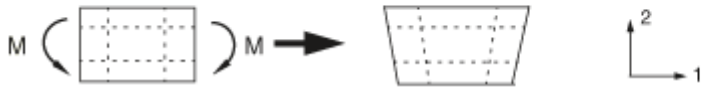
Figure 4–6 Deformation of a fully integrated, quadratic element subjected to bending moment M .
